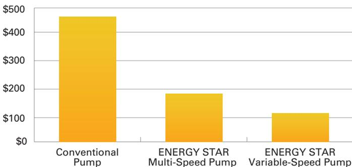
Two-speed models use a low speed for filtration and a high speed for cleaning, reducing pump electricity use by up to 50 percent. Variable-speed models alternate between slow and fast modes to deliver the right flow for different tasks, reducing pump electricity use by up to 75 percent.
